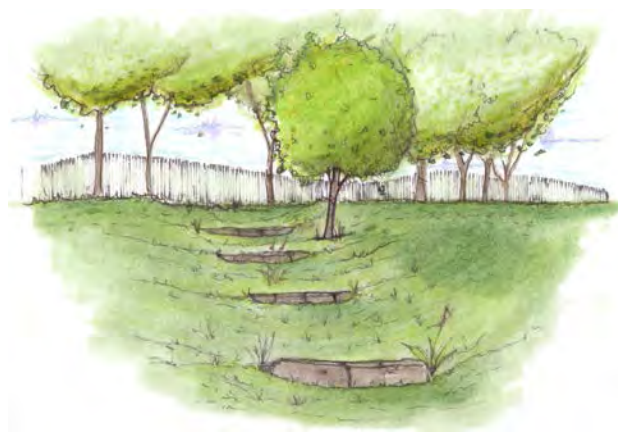
Figure 2. Check dams within a swale slow the flow, allowing sediments to settle out and some infiltration to occur.
