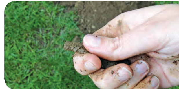
Figure 1 – Soil ribbon test.
